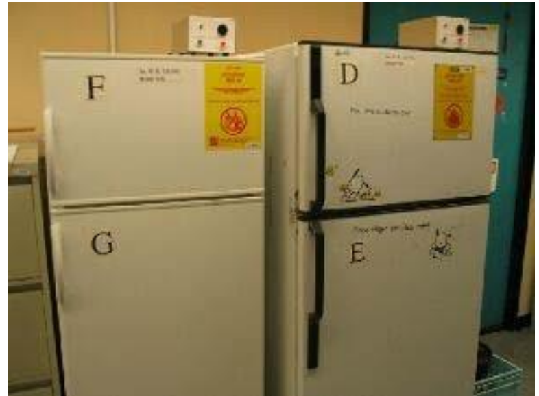
Explosion-proof Refrigerator: Storage of hazardous chemical
